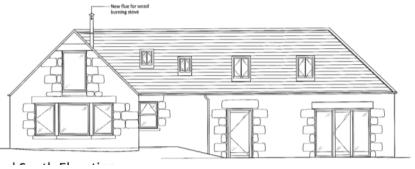
Proposed elevations showing additional velux windows and flue
